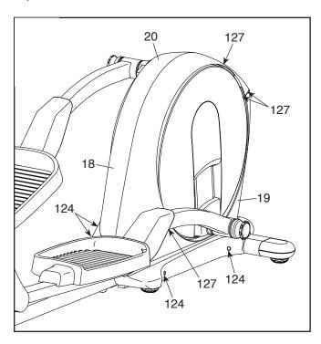
Next, remove the M4 x 16mm Round Head Screws (127) and the M4 x 42mm Screws (124) from the Right and Left Shields (18, 19). **Make sure to note which size of Screw you remove from each hole.** Then, gently remove the Left Shield.
